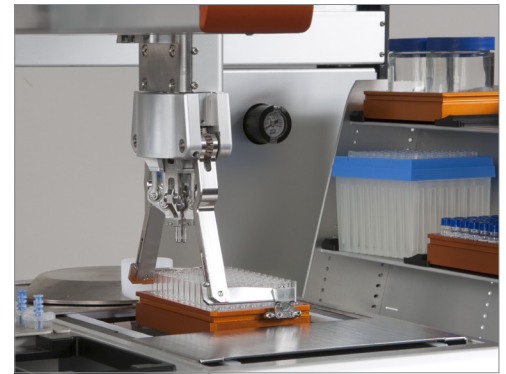
CM Protégé delivering a plate from the integrated shoulder hotel to the balance.
